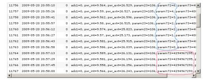
You can see that when temperature goes down and crosses 0 degrees threshold the necessary negative numbers are constituted with enormously large ones.
