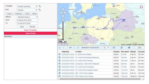
If the text in a cell is blue, it means that there are coordinates for this point. Click on such a cell to move to that place on the map.
