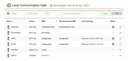
To add a new unit to the retranslator, give it a name, indicate device type, IMEI (unique ID) and retransmission IMEI. For existent units, not only these parameters are displayed but also time of last received message and status (being retransmitted or not). Any of these parameters can be used to sort the list of units. Besides, to quickly find a unit, you can use the dynamic filter by name.
