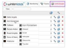
⋄ or ⋄ — Edit or view unit group properties – depends on your access (change name, add more units, remove units, manage access, etc.). The dialog of unit group properties can contain up to 4 tabs which were described above:
